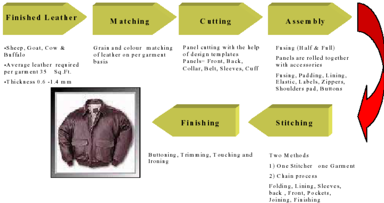
Figure - 1 Process Flow for Leather Garments Manufacturing
